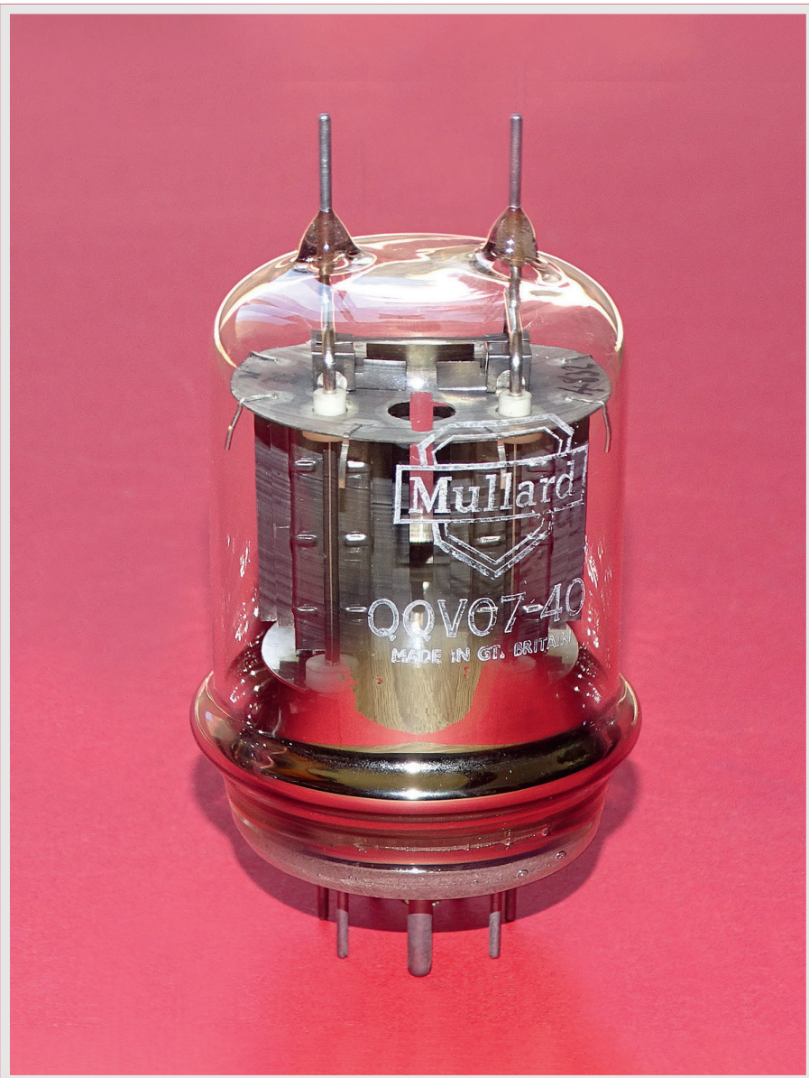
The QOV07-40 (829B) push-pull beam power tetrode was popular as a 2m power amplifier. It can deliver an output of over 85W.
