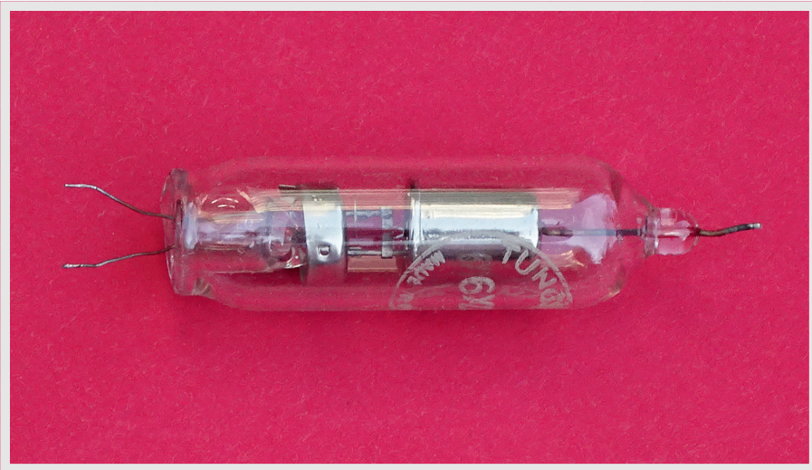
50 years after Fleming's valve, diode vacuum tubes were still useful as high voltage rectifiers. This 6X2 can support a peak inverse voltage of 17kV.
