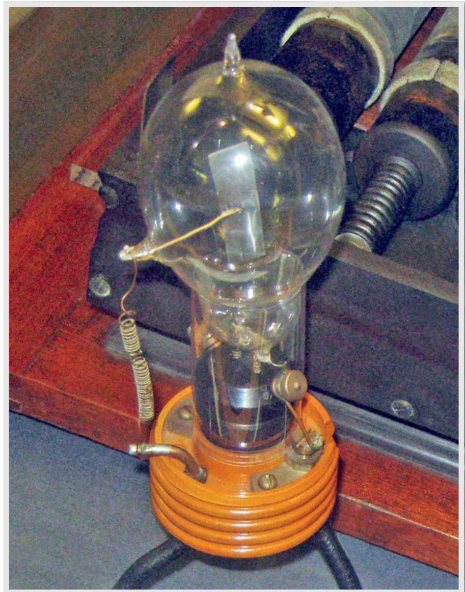
Experimental diode valve used by Ambrose Fleming for early experiments, and in 1904 for radio signal detection.
