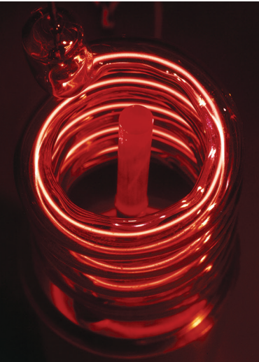
Maiman's original laser was based on a ruby crystal within a coiled xenon flashtube.
