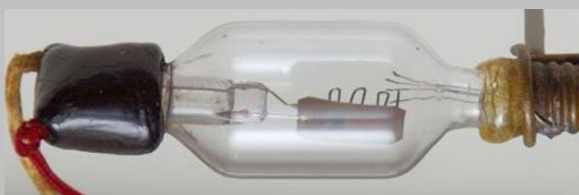
Audion Tubular / Tubular Audion.
