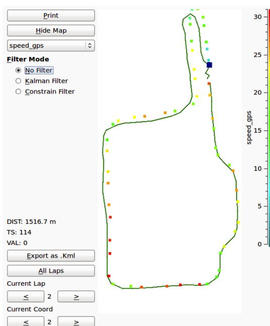
Figure 6.10: Acquired coordinates without any filtering.
