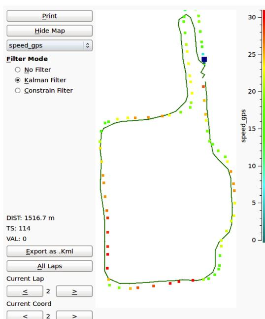
Figure 6.11: Acquired coordinates using Kalman filter.
