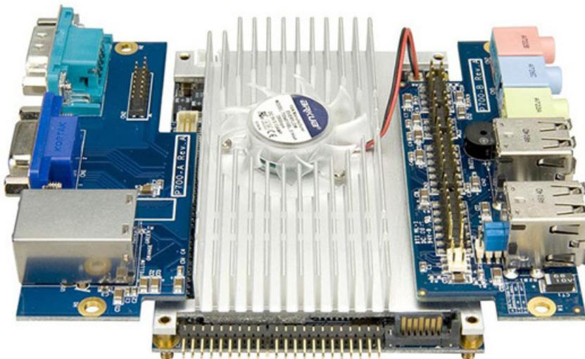
Figure 4.1: VIA EPIA-P700 Board equipping the car's station [6].
