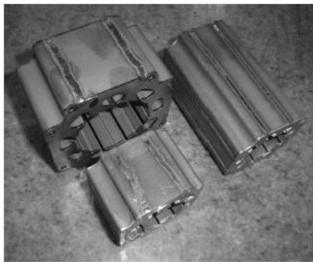
Figure 2.11: Stator welding as a stacking method [4].
