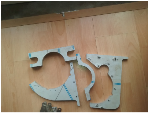
(a) Support pieces after waterjet cutting.
