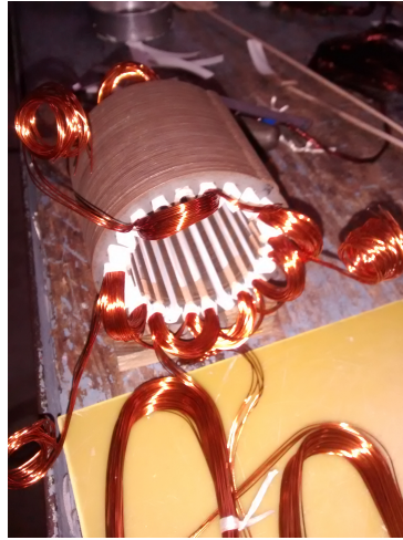
Figure 4.5: Winding carried out by Lehmus.
