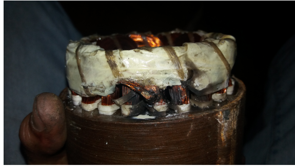
(b) Winding phase damage.
