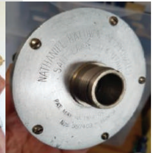
Baldwin loudspeaker transducer
