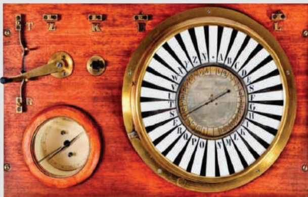
Siemens & Halske – Telegraphic Pointer- 1846.
