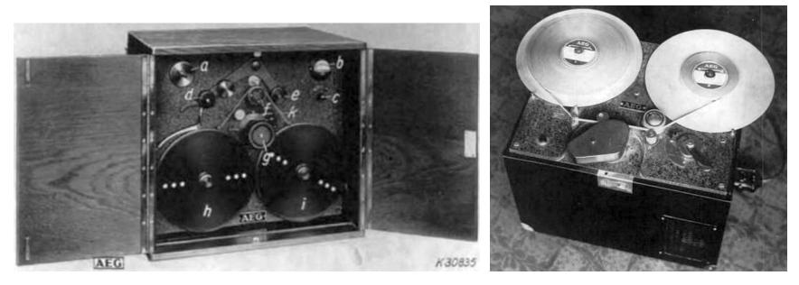
1935 - AEG 4<sup>th</sup> prototype introduce the play disc style and pancake style of plates to support tape; this will be a standard in professional audio
