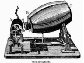
*BC*, barrel with opening at  $C_i$ ,  $c_i$  brass tube with membrane and style at  $\delta_i$  and movable piece  $a_i$  by which the position of the nodal points can be regulated i  $k_i$  handle to turn cylinder (*A*) covered with lampblacked paper.
