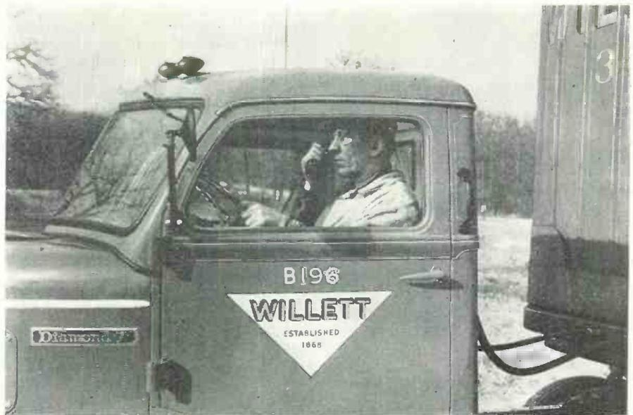
Willett truck driver contacts his dispatcher over two-way radio installed in vehicle.
