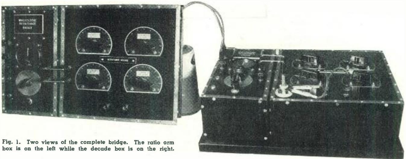
Fig. 1. Two views of the complete bridge. The ratio arm box is on the left while the decade box is on the right.
