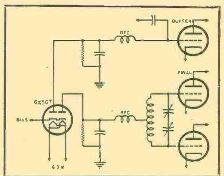
If the grid current greatly exceeds the supply rating, and the grid leak draws a small current, bias isolating rectifiers may be used. The grid leak values will depend on the type of tube in use.
