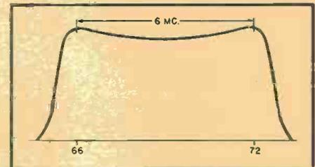
Fig. 6. Alignment r.f. curve (channel four).
