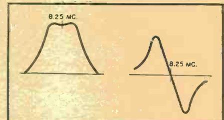
Fig. 7. Sound channel alignment curves.
