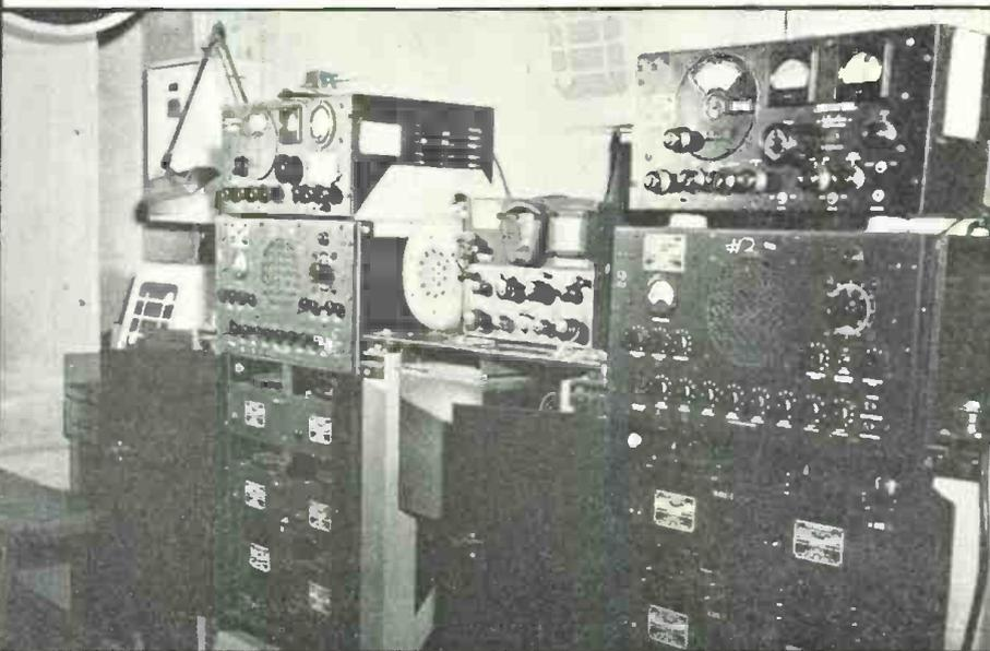
Hallicrafters S-27 and S-26 receivers aboard the Shangri-La were used to feed programs, etc. to 20 ship's speakers, or record communications on 12 transcribers.
