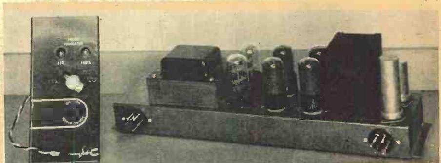
(Left) Neon volume indicator. (Right) 30 watt booster unit for amplifier.
