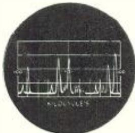
**THE STAGE WAS SET!** At approximately 11:30 P.M. the British Broadcasting Company and a Spanish station were still to be seen and heard on the 40 meter band. Their signals occupied the center of the screen. On the edge of the screen, but outside of the band, were a few cw and phone stations.
