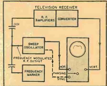
Fig. 5. Alignment diagram for r.f.
