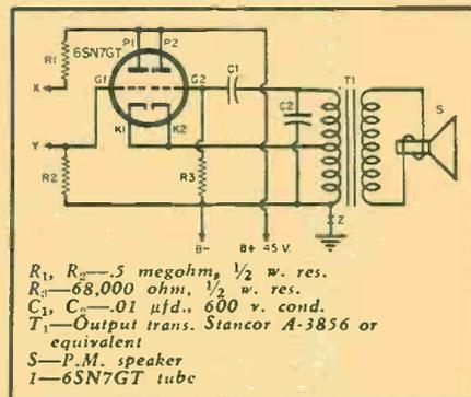
Fig. 1. Circuit diagram for control tube keyed audio oscillator.
