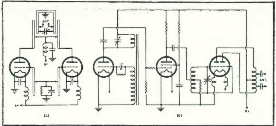
Fig. 4. Conventional diagram of two types of metal locators.
