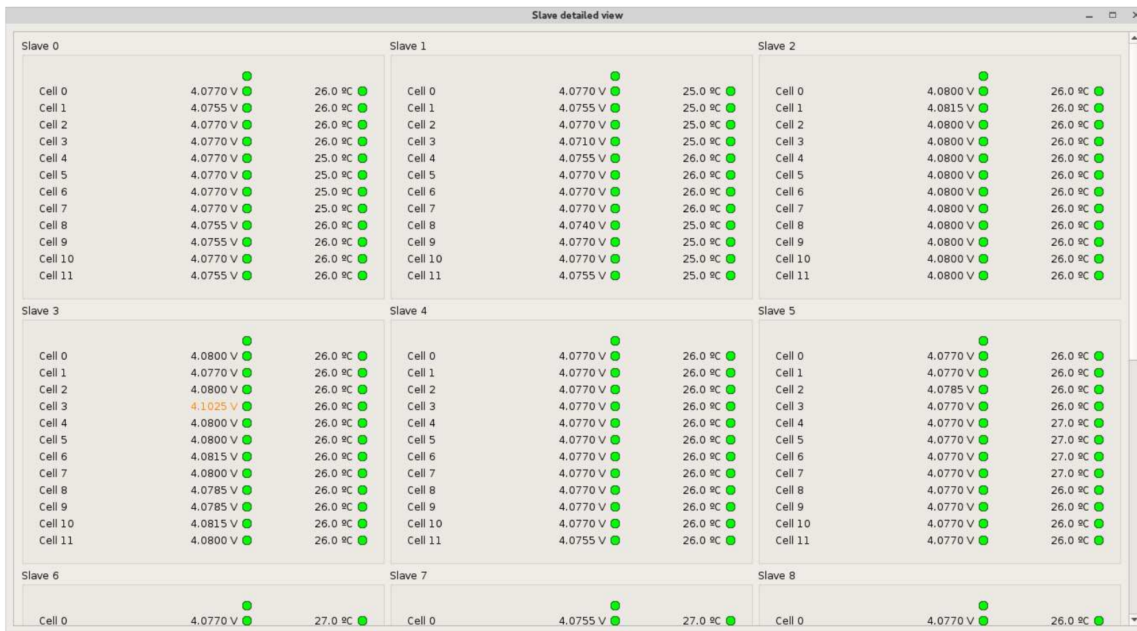
Figure 7.5: Cell voltages in a final stage of balancing. Green 'lights' indicate good connections to cells and sensors.
