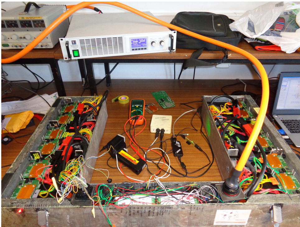
(b) Charging test. Special connector emulates a number of the car's systems. LED (bottom left) indicates high voltage.
