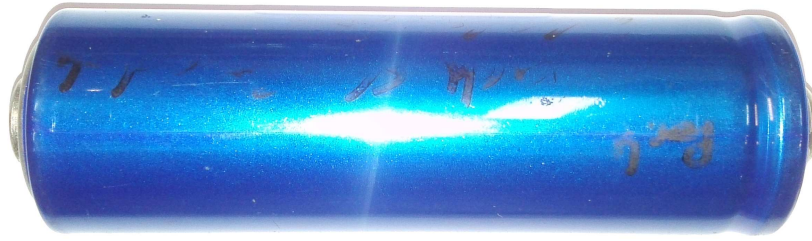
(a) Headway 38120S cylindrical lithium-ion cell, as used in FST-04e (120×38mm).
