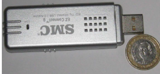
Figure 2.12: Wi-Fi USB device installed on the mobile station [7].
