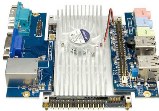
Figure 2.8: VIA EPIA-P700 Board equipping the car mobile station [7].
