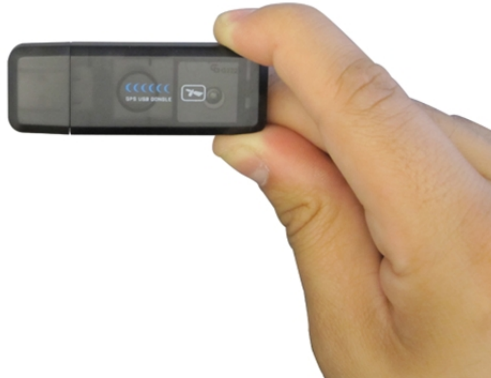
Figure 2.11: Supporting GPS device installed in the mobile station [8].
