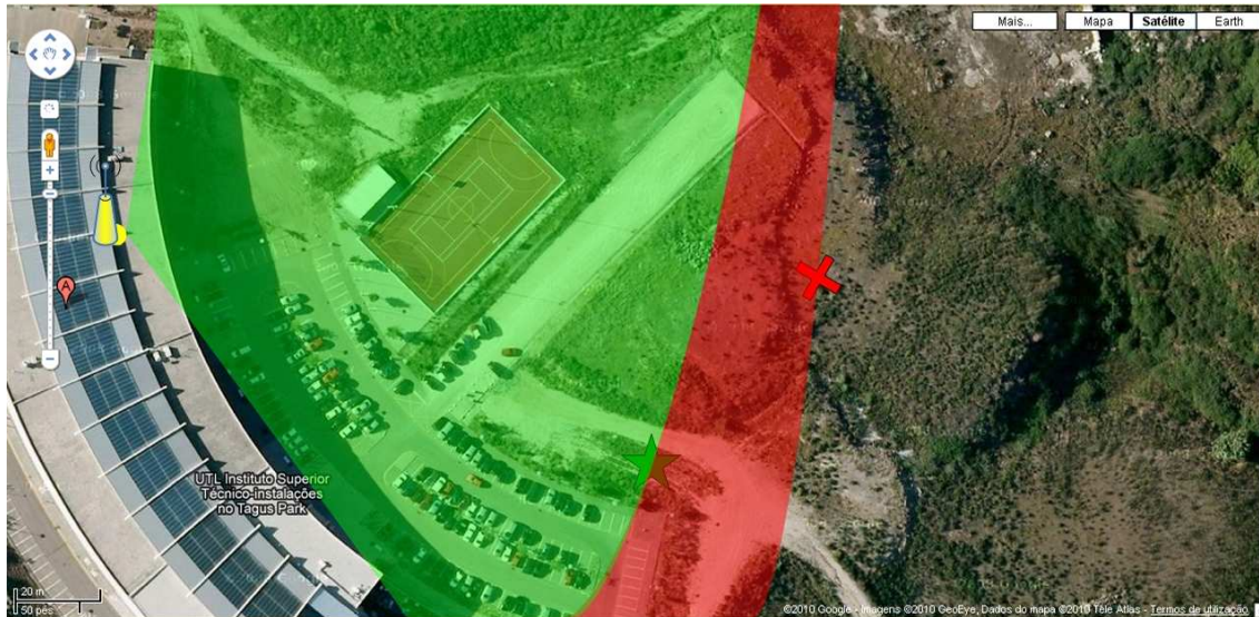
Figure 7.1: Testing area of the communication system: the green zone denote places where there is acquisition of signal; the red zone is where the signal is lost.
