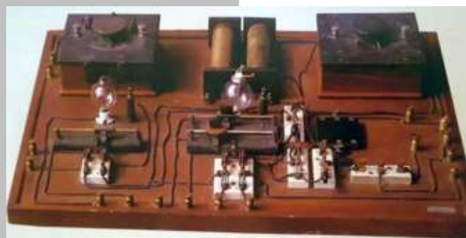
Roy Weagant Radio Detectors Left – With Fleming Diode; Right – With Forest Audion
