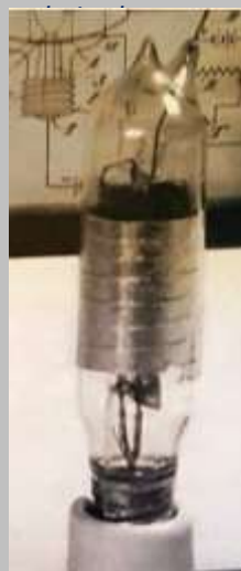
Audion With external grid / Com grelha externa
