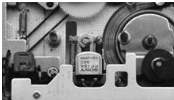
Fig. 6.17. TCM-280 erase head, recording/playback head
