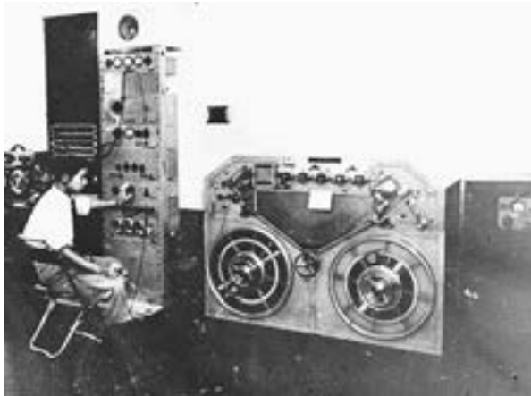
Fig. 3.10. Marconi-Stille steel ribbon recorder (1937) (9)
