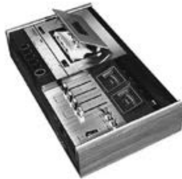
Fig. 11.5. Cassette deck with inbuilt Dolby B system TEACA-350 (1971)
