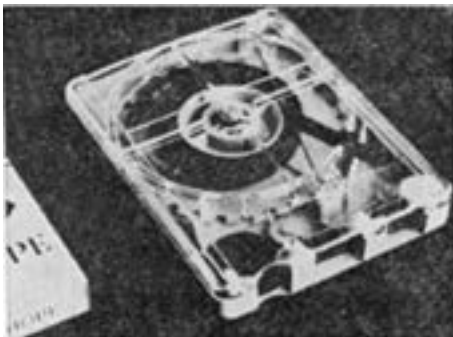
Fig. 6.3. Fidelipac cartridge (1962) (3) 102 x 133 x 24 mm four-track/two channel
