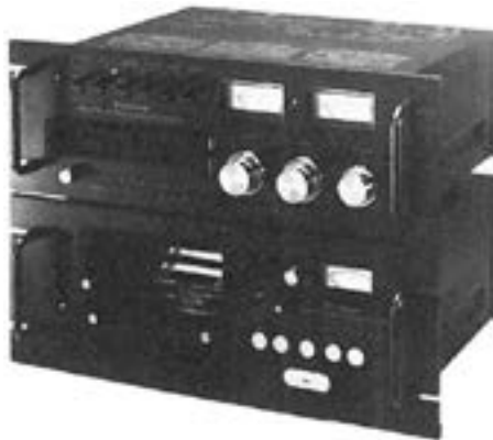
Fig. 10.5. Matsushita RS-690 (1975) (4) Mechanism and amplifier are separate
