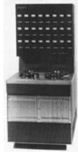
Fig. 14.5. Sony 24-channel stationary-head DAT prototype (c. 1977) (4)
